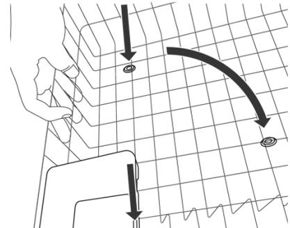
3. Let the rack down completely; the rack will lock itself into the holders:
